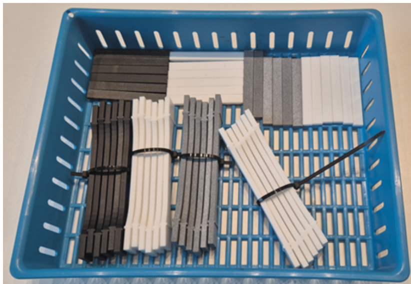
Figure 2 - Example Sample Segregation for Sterilisation Cycles, white coloured parts were for this investigation
